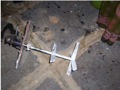
Fig. 2: Light duty (for 15 liter DDU) and heavy duty (for 100 liter DDU) electric stirrers used in Yellodu village
