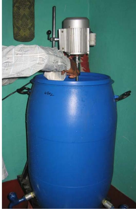
**Fig. 2:** Light duty (for 15 liter DDU) and heavy duty (for 100 liter DDU) electric stirrers used in Yellodu village
