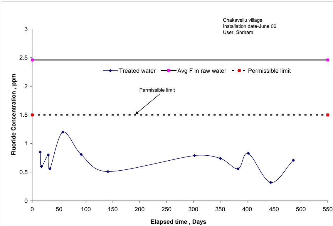
**Fig. 6:** Variation in fluoride concentration in treated water samples as function of treatment period: 15 liter DDU with electrical stirrer
