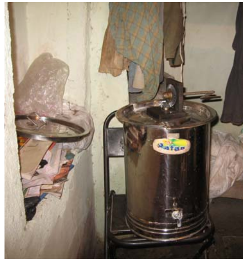
Fig. 3: DDU with mechanical (hand-operated) stirring device used in Chakavellu village
