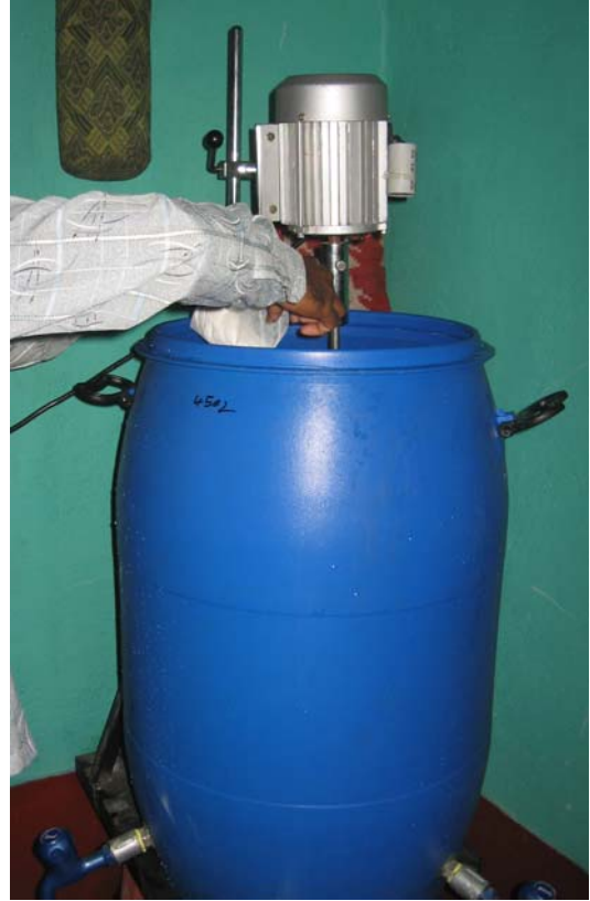
Fig. 2: Light duty (for 15 liter DDU) and heavy duty (for 100 liter DDU) electric stirrers used in Yellodu village
