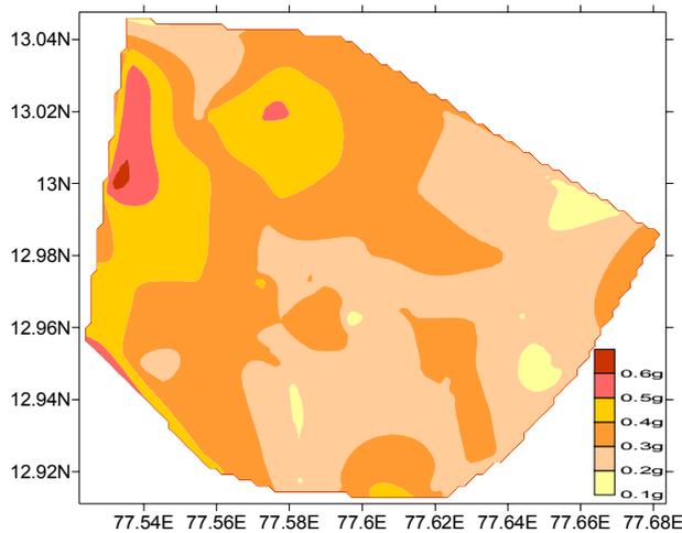
Fig. 15 Peak Ground Acceleration Map at Ground Level of Bangalore
