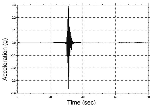
Fig. 13(a) Acceleration time history at ground surface
