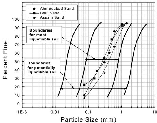
Fig. 1 Grain size distribution of soils used in this study along with soils tested along with soils susceptible for liquefaction proposed by Tsuchida (Iwasaki, 1986)
