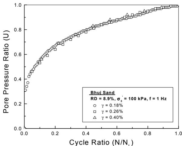
Fig. 3 Relationship between normalized pore pressure ratio and cycle ratio for Bhuj sand of RD = 8.9% and various shear strains
