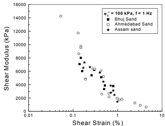
Fig. 9 Variation of Shear modulus and shear strain for Bhuj, Ahmedabad and Assam sand
