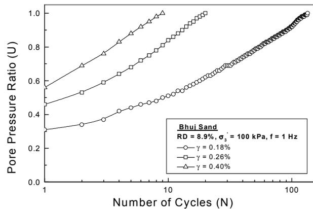
Fig. 2 Pore water pressure build up as a function of number of cycles for Bhuj sand for RD = 8.9% and various cyclic shear strains
