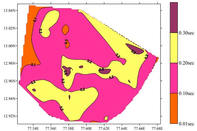
Fig. 16 Variation of period of the soil column at various locations
