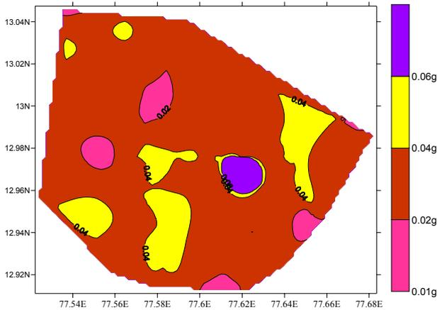
Fig. 17 Spectral Acceleration Map of Bangalore at 1.5 Hz Frequency
