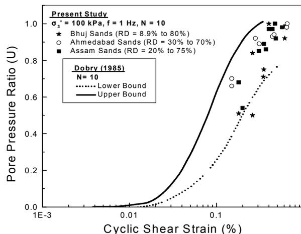
Fig. 5 Relationship between pore pressure ratio and cyclic shear strain for Bhuj, Ahmedabad and Assam sands
