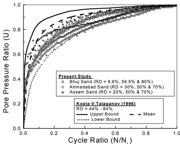
Fig. 6 Comparison of pore water pressure generation in Bhuj, Ahmedabad and Assam sands for different relative densities in strain-controlled tests
