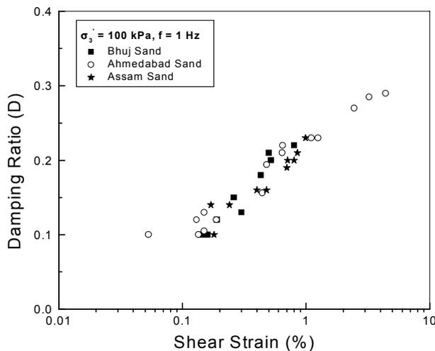
Fig. 10 Variation of Damping ratio and shear strain for Bhuj, Ahmedabad and Assam sand
