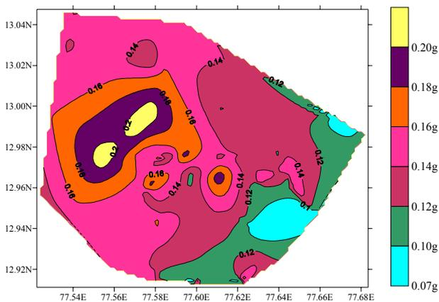
Fig. 12 Peak Acceleration Map at Rock Level
