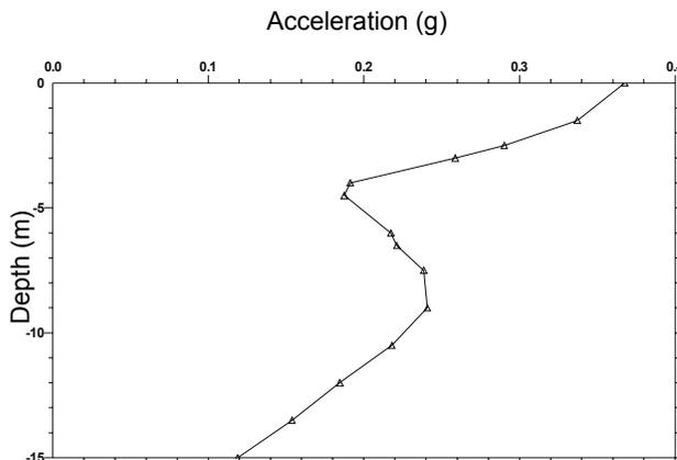
Fig. 13(b) Variation of peak acceleration with depth
