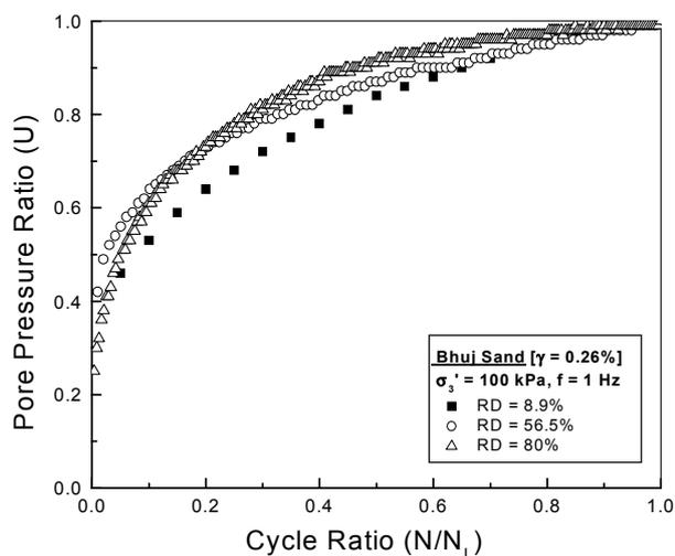
Fig. 4 Relationship between normalized pore pressure ratio and cycle ratio for Bhuj sand of RD = 8.9, 56.5 & 80% and shear strain of 0.26%
