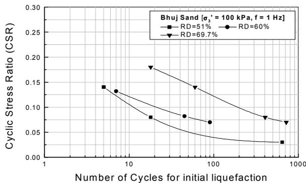
Fig. 7 Variation of cyclic stress ratio with number of cycles for initial liquefaction of Bhuj sand
