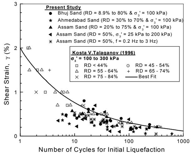
Fig. 8 Relationship between shear strain and number of cycles for initial liquefaction for Bhuj, Ahmedabad and Assam sands
