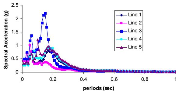
**Fig 10: Response Spectrum at surface using MASW**
