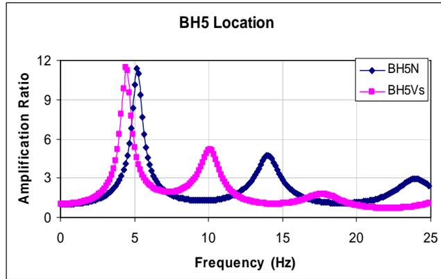
Figure 15: Amplification Ratio with Soil Column Thickness
