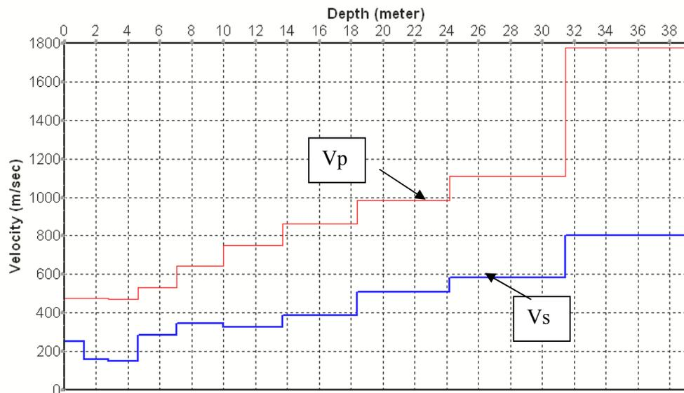
**Figure 4: Typical  $V_s$  and  $V_p$  Plots for Line 1-1**
