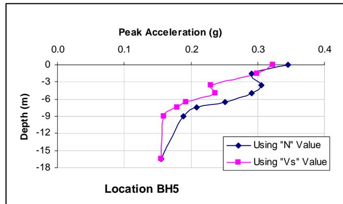
Figure 12: Peak Ground Acceleration with Soil Column Thickness
