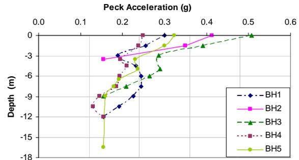
**Fig 9: Peak Acceleration with depth using MASW**
