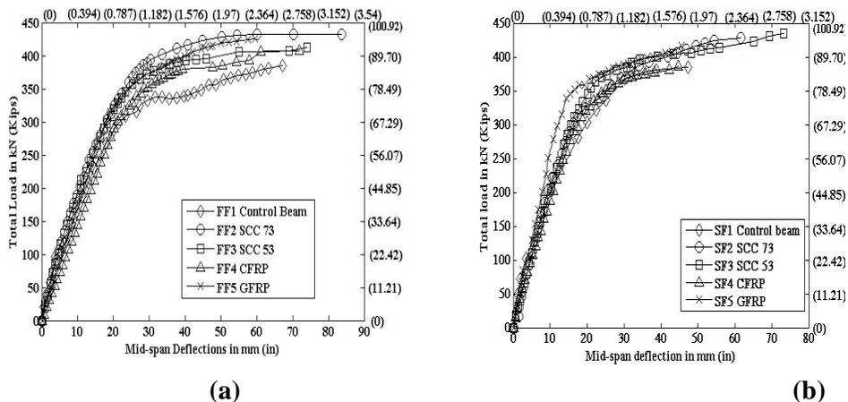
**Figure 14: Load versus deflection of (a) flexure repaired and (b) shear repaired beams**
