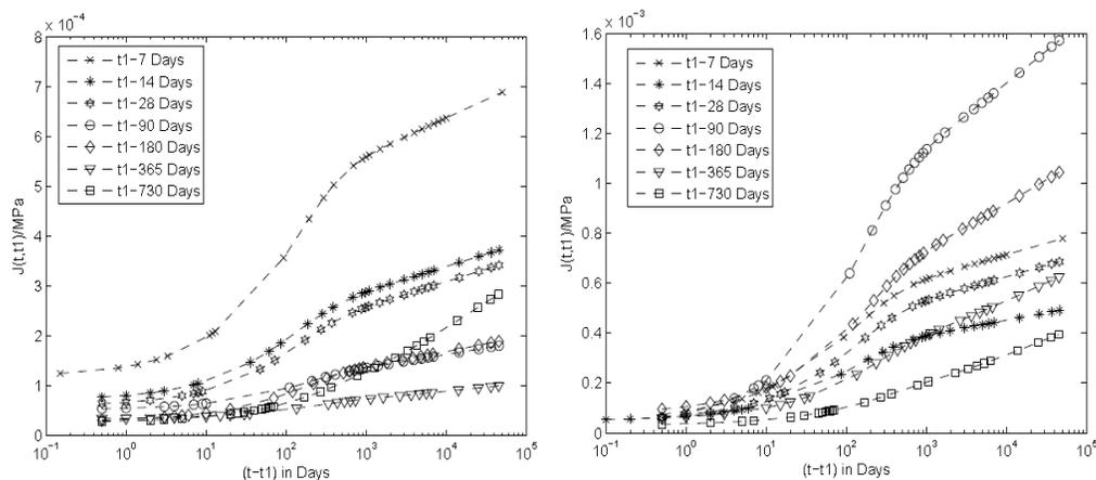
**Figure 13: Long term creep prediction using short term data for normal and heavy density concrete**
