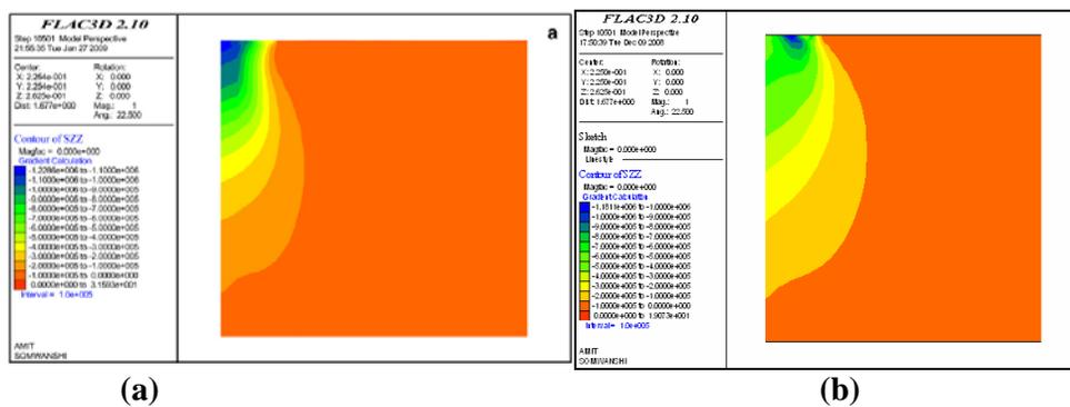
**Figure 31: Vertical stress distribution below footings on reinforced sand beds (a) planar reinforced (b) geocell reinforced**
