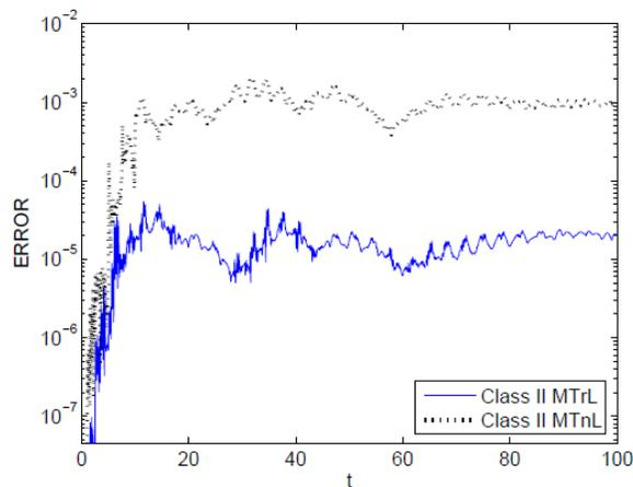
**Figure 25: Lesser error propagation via (a version of) the transversal linearization (MTrL) vis-à-vis (a similar version of) the tangential linearization (MTnL); the dynamical system is a nonlinear 3-DOF oscillator**
