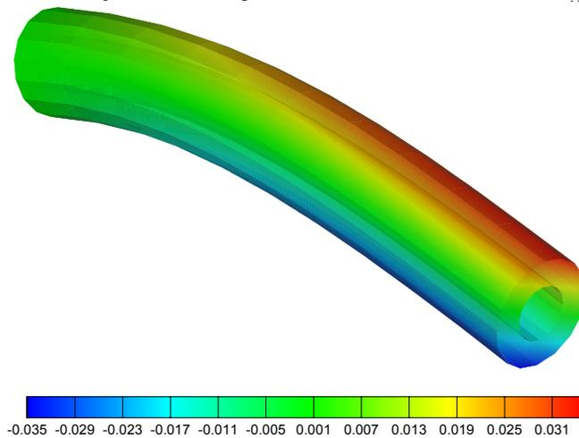
**Figure 27: NURBS-based approach bridging mesh-free and finite element methods: horizontal displacement profile of the hollow cylinder**
