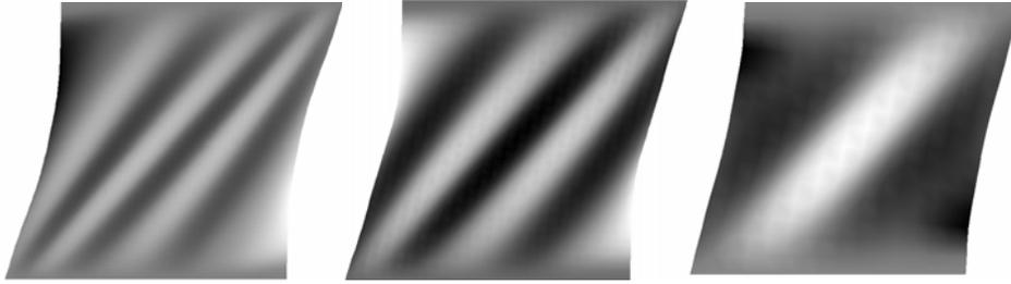
**Figure 28: Cosserat point solution for out-of-plane deformation of an ultra-thin membrane using a regularized form of 3-D nonlinear elasticity equations; (left) 2500 Cosserat points; (middle) 900 Cosserat points; (right) 100 Cosserat points**
