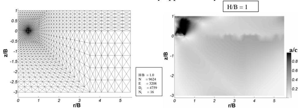
Figure 33: Finite element mesh & failure patterns for circular anchors in clays, whose cohesion increases with depth, under vertical uplift.
