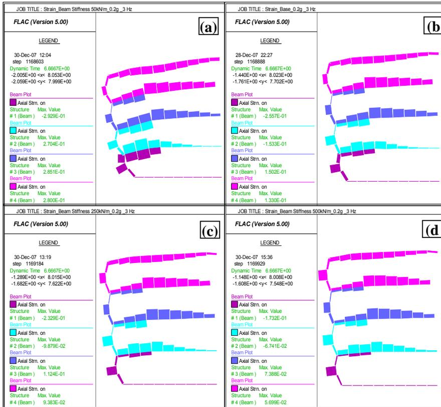
Figure 32: Axial strain distributions along the reinforcement elements in retaining wall for stiffness values: (a) 50 kN/m, (b) 150 kN/m, (c) 250 kN/m and (d) 500 kN/m
