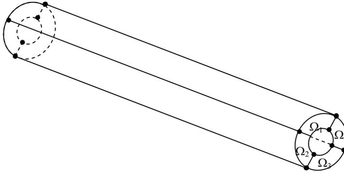
**Figure 26: NURBS-based approach bridging mesh-free and finite element methods: discretization of a hollow cylinder into just four elements (or sub-domains)**
