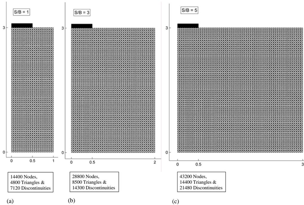
**Figure 30: Finite element mesh for (a)  $S/B = 1.0$ ; (b)  $S/B = 3.0$  and (c)  $S/B = 5.0$**
